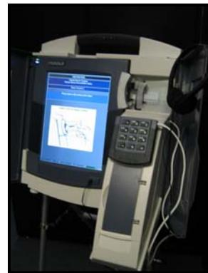
**STEP FOUR**—Congratulations! You finished setting up your TSX unit! If you are using a VIBS kit with this unit, clip the keypad to the outside of the printer module cover and verify that the headphones are plugged in. Also, don't forget to record the statistical information from the bottom of the screen on the *TSX Periodic Check Sheet for Election Day*.
