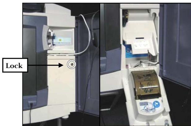
**STEP ONE** — Unlock and open the printer door. Observe unit’s internal printer and its components. If not using the AVPM, leave this door locked. The set up is complete.
