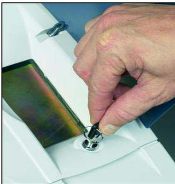
**STEP ONE** — Unlock and raise the printer housing cover.
