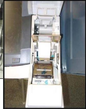
**STEP SEVEN** — Place a new roll of paper in a plastic spool and slide it into the center of the printer housing. When inserted in the unit, the paper should sit so the end of the paper comes out from the bottom of the roll and the large end of the spool is on the left hand side.
