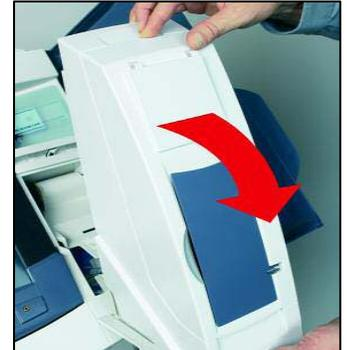
**STEP FOUR** — Locate the white latch at the top of the printer housing. Pull it to release the printer housing from the TSX Unit. Close the printer housing cover and remove it from the TSX Unit.
