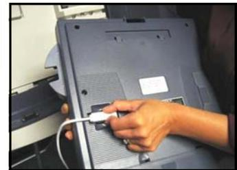
**STEP ONE** — With the privacy panels opened, find the black button on top of the tablet. Press the button and pull the tablet towards you. You will now be able to see behind the tablet.
